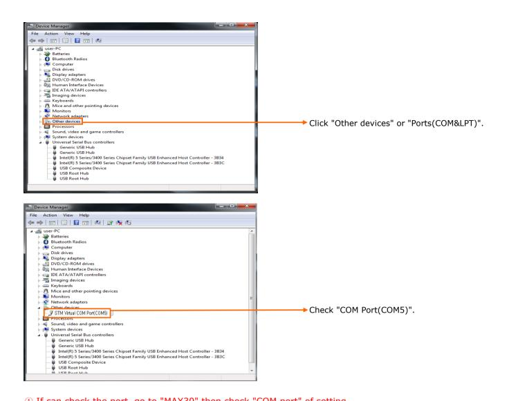
① If can check the port, go to "MAX30" then check "COM port" of setting.
