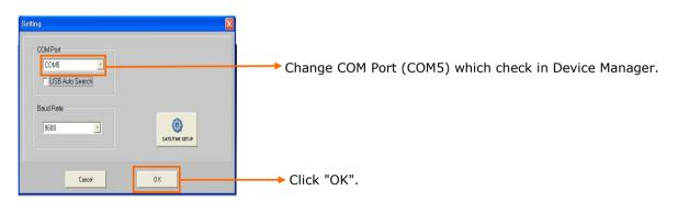
② If not working with above procedure, please refer to an installation guide and re-insall the driver.
